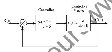
2.a) Determine the overall transfer function relating C and R for the system whose block diagram is given in figure.
