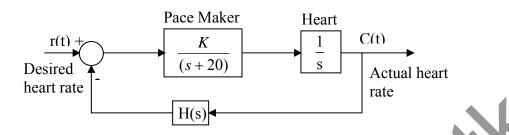
Determine the sensitivity of the closed loop system transfer function to small changes in K at the normal heart rate of 72 beats per minute if H(s) = 1 and the nominal value of K = 400.
